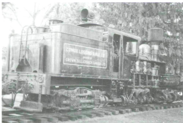
Fig. 4. A representative Shay locomotive. This machine is Lima No. 3311, a typical, modern two-truck Class B Shay. Preserved at Ladysmith, B.C., by Crown Zellerbach Canada. (Photo: BCPM, uncatalogued.)
