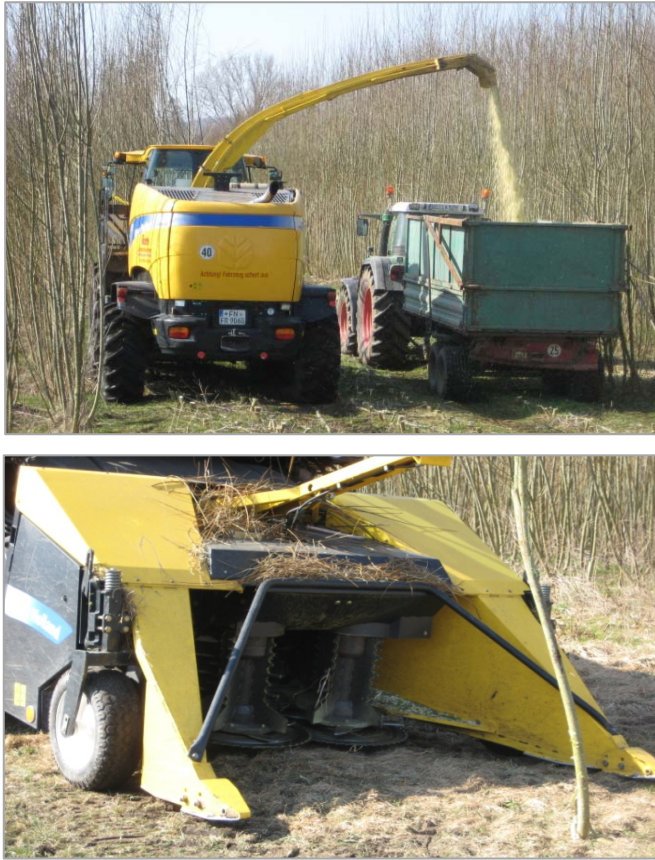
Figure 1. New Holland FR 9060 while harvesting 3-year-old willows in double-row system (top) and cutting head 130 FB (bottom). Photo: Janine Schweier.
