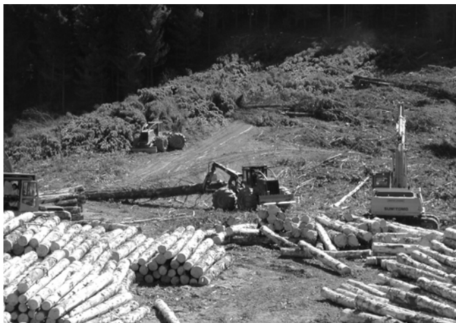
Figure 2. Mechanised processor located more centrally on the landing to minimize fleeing distance.
