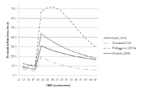
**Figure 6.** Dangle-head processor felling and processing production rate comparisons.
