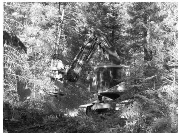
Figure 1. ~ TigerCat L830 tracked, swing-to-tree feller-buncher with a 5400 series 22-inch DBH capacity felling head felling small trees.
