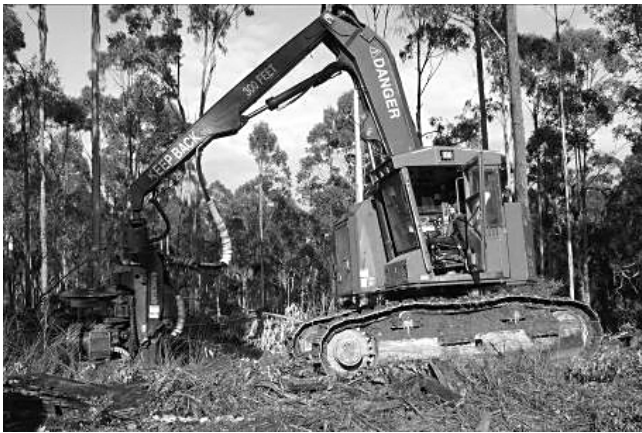
Figure 1. ~ Single-grip harvester "Timberjack" 608S – (harvester-processor or processor only).
