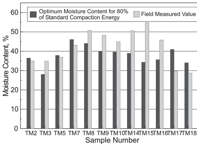
**Figure 3.** ~ Comparison between optimum moisture content for 80% of standard compaction energy and field moisture content at time of construction.
