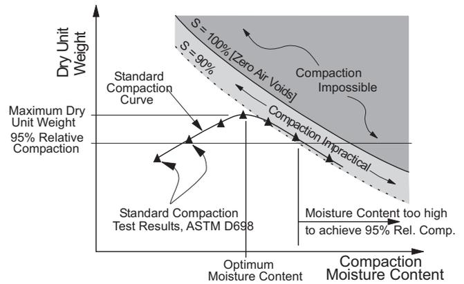
**Figure 4.** ~ Schematic relationship between field MC, saturation, dry unit weight, and standard compaction test results.
