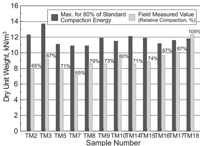
**Figure 2. ~ A comparison between the maximum dry unit weight for 80% of the standard compaction energy and field dry unit weight of subgrade materials along the test road (field measured dry unit weight bars are labeled with relative compaction values for completeness).**
