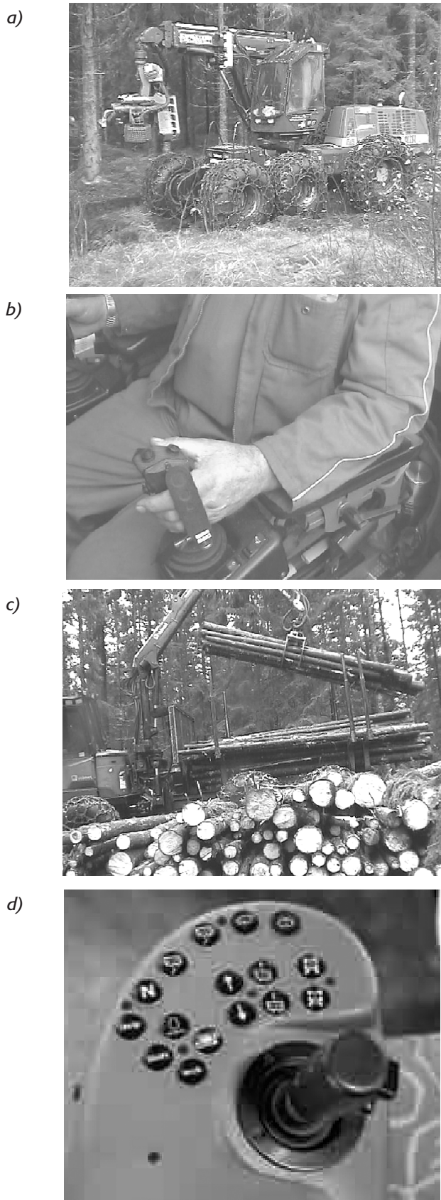
Figure 2. ~ Valmet harvester with the crane on the right side of the cabin (a) and the accompanying control lever and VDU display (b); Valmet forwarder (c) with the control lever (d).
