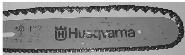
Figure 3. ~ The standard saw-bar with a saw-chain without cutting teeth.
