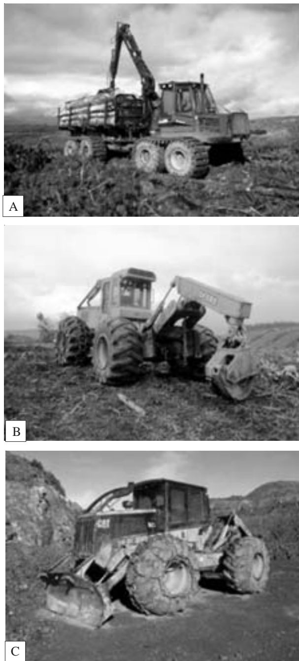
Figure 1. Machines used in the study: (a) Timberjack 1710 forwarder, (b) John Deere 648G-II skidder, (c) Caterpillar 525 skidder.
