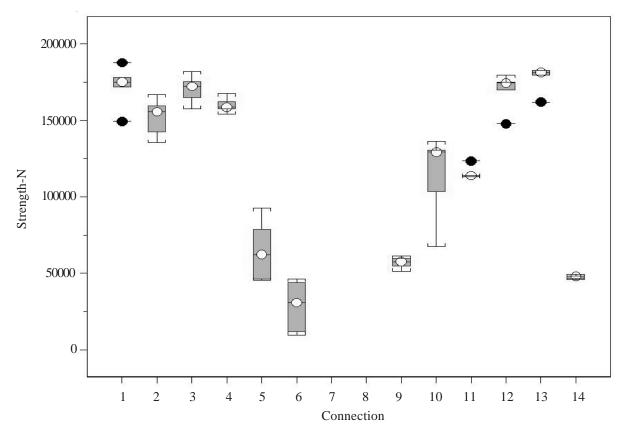
Figure 7. Boxplot of 14mm diameter performance. *Spliced* end connections numbered 1-4, *Adhesives* 5, 6, 9, 10, *Dry Hardware* 11-14. End connections 7 and 8 omitted in testing of this diameter class.
