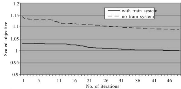
Figure 13. Scaled objective function value for two scenarios, one with and one without train system.
