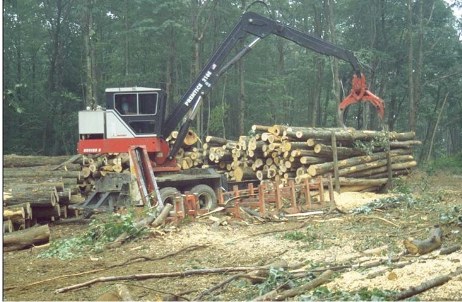
Figure 1. Loader with saw-bunk and measuring rack.
