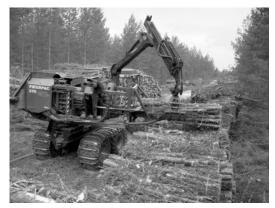
Figure 2. Bundling tree sections at the roadside landing.
