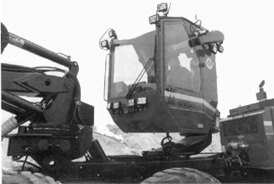
Figure 1. The self-leveling and swiveling cab suspended from an arched column attached to a swiveling socket.
