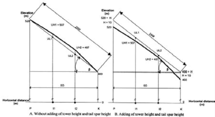
Figure 5. Modelling of skyline skidding distance, cut profile.
