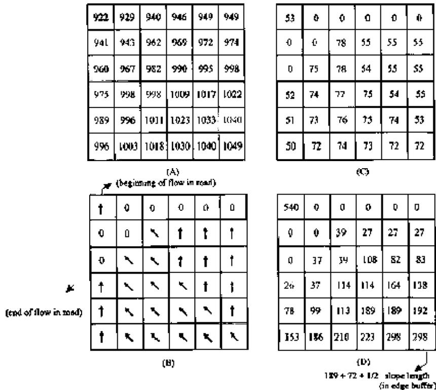
Figure 2. (A) Grid representing DTM (resolution 50 m); (B) Flow direction = direction in maximum downhill slope; (C) Slope length calculated from maximum downhill angle; (D) Cumulative slope length.
