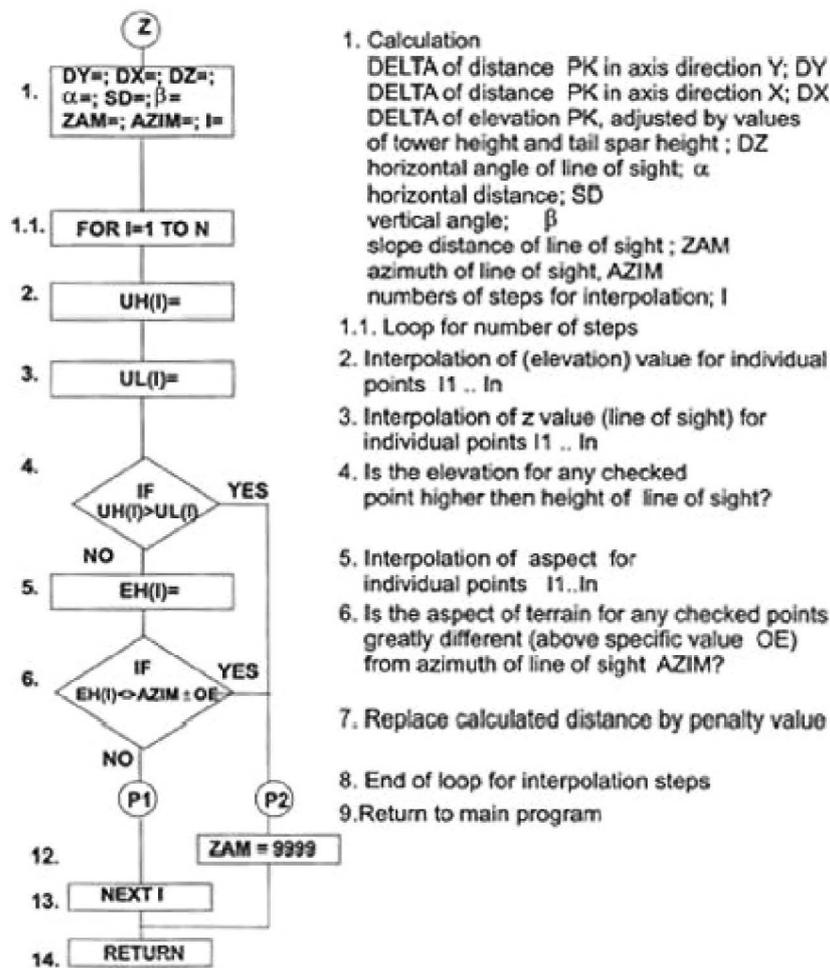
Figure 3b. FLOWCHART - Modelling of skyline skidding distance.
