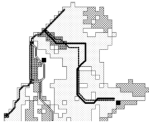
Figure 6. A single road route determined by dynamic (solid) and heuristic (dashed) programming.
