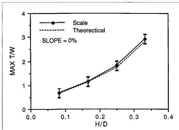
Figure 8. Comparison of maximum towing forces for a vehicle with rigid wheels, theoretical versus scale model.
