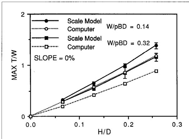
**Figure 10.** Comparison of maximum towing force results for a vehicle with pneumatic tires, computer simulation versus scale model.
