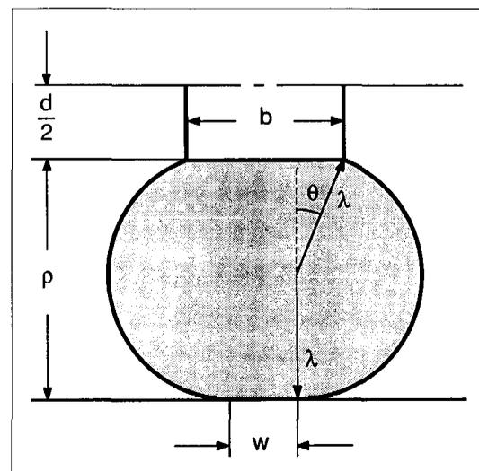
Figure 6. Radial cross section of deflected tire.
