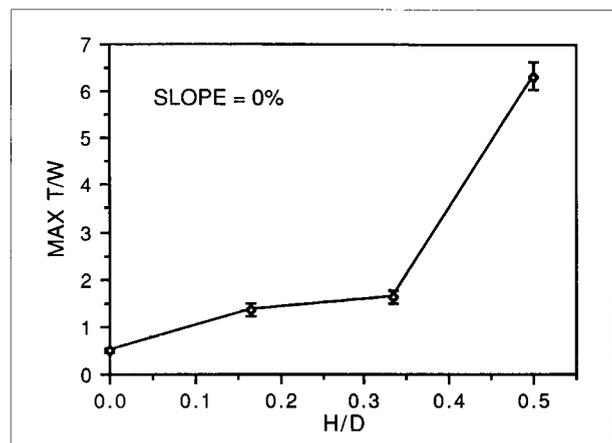
**Figure 13.** Maximum towing force results from scale modeling for a vehicle with rimless spoke wheels, with slope = 0 percent.
