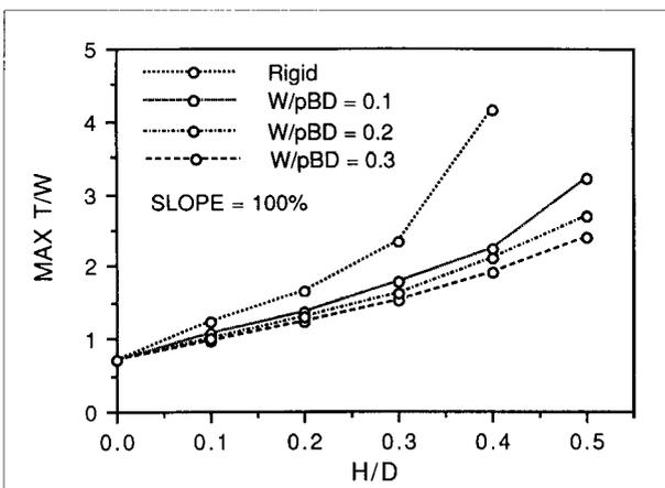
**Figure 12.** Maximum towing force results from computer simulation for a vehicle with pneumatic tires, with slope = 100 percent.
