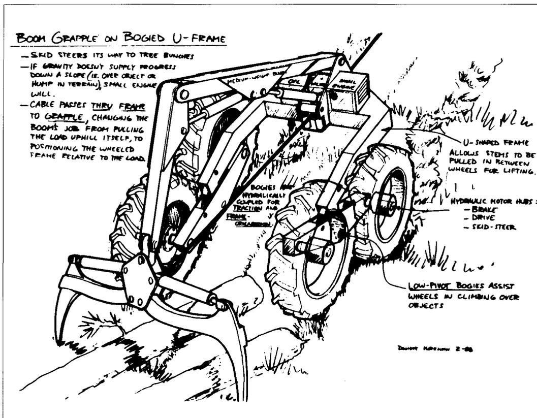
Figure 1. Cable-towed vehicle concept.
