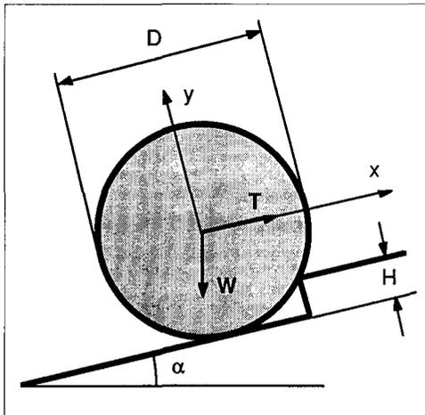
**Figure 2.** Obstacle and wheel geometry and forces.
