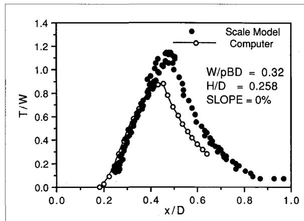
Figure 9. Comparison of towing force traces for a vehicle with pneumatic tires, computer simulation versus scale model.
