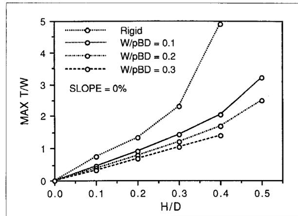
**Figure 11.** Maximum towing force results from computer simulation for a vehicle with pneumatic tires, with slope = 0 percent.
