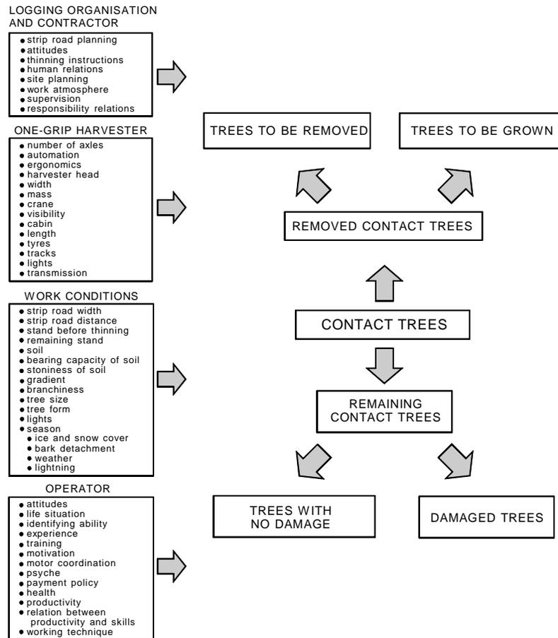
Figure 1. Elements influencing tree damage in a one-grip harvester operation.
