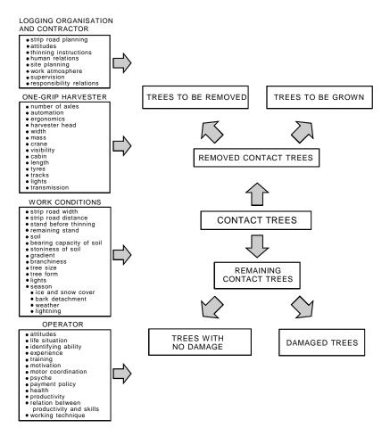
Figure 1. Elements influencing tree damage in a one-grip harvester operation.
