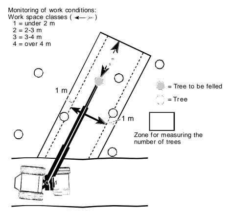
Figure 2. The method of estimating the available space and number of trees on a machine's working area.
