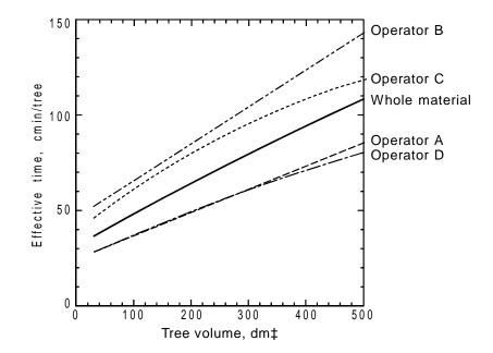
Figure 4. The influence of stem size on effective time consumption with spruce by operator.
