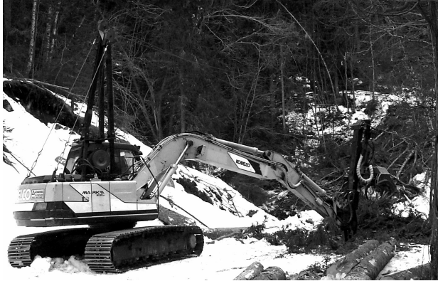
Figure 6. Stability was provided by boom support on the ground. The machine had no stability problems during the extraction operation.
