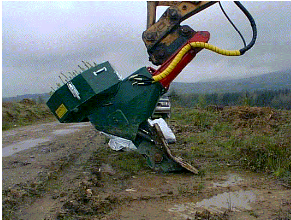
Figure 1. The Bräcke planting machine.
