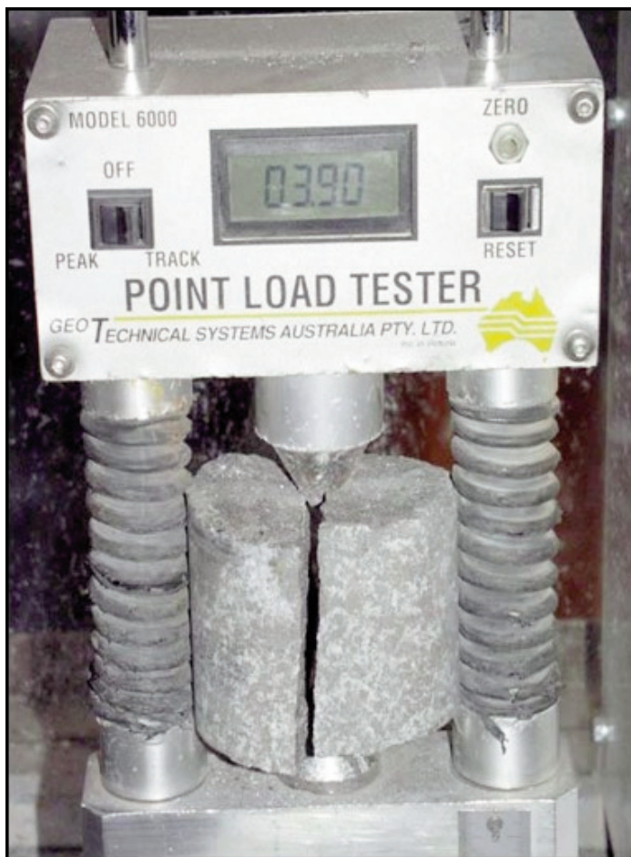
Figure 3. Example of point load testing of drill core. (image from Kojovic 2008). Force applied to the rock is gradually increased until the rock fails. The peak pressure applied is shown on the gauge.
