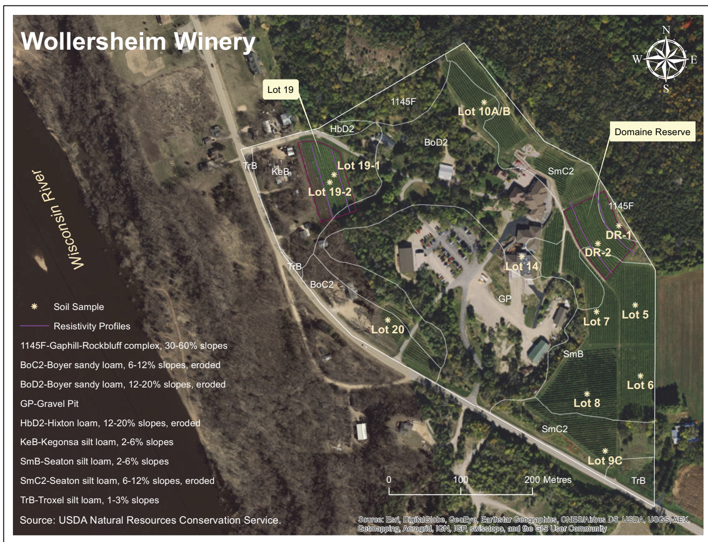
Figure 4. Location map of Wollersheim Winery vineyards illustrating the distribution of soil types, and soil sample and resistivity profile locations.
