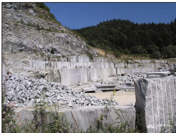
Figure 2. Active quarry in granodiorite near the village of Cezlak. Photo: Samo Jenčič.
