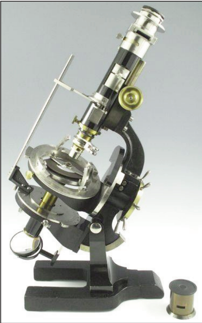
Figure 1. Petrographic microscope with a universal stage (Kile 2009).
