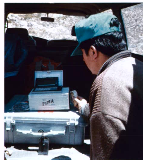
Figure 8 PIMA (Portable Infrared Mineral Analyser) at use in the field. Anne Thompson of PetraSciences Inc. was the MAP course instructor in PIMA training sessions conducted for geologists from participating countries (photo by A. Thompson).
