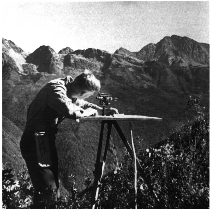
Figure 5 Geologist J.G. (Jim) Fyles surveying by plane table near Zincton in the Kootenays, 1948 (M.S. Hedley).
