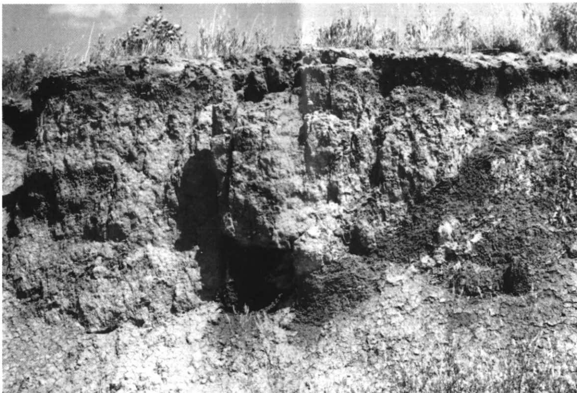
Figure 8 Brunisol developed on loess over Pleistocene-aged lacustrine silts, Peace River Valley, British Columbia. Abundant salt efflorescence is present on the surface. Pedology is very much a part of the larger picture of the earth sciences. Sections such as this reveal much about the nature of climates under which the soils have been formed (M. Church).
