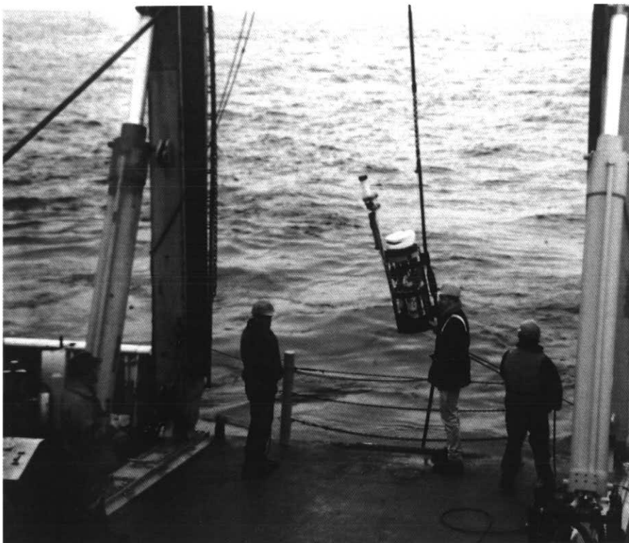
Figure 6 Deploying a sample cluster in oceanographic work (S.E. Calvert).
