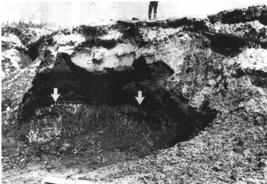
Figure 2 Exposure showing permafrost table (arrowed), underlying frozen silts (permafrost) and overlying supra-permafrost layer that freezes in winter and thaws in summer. Figure for scale.
