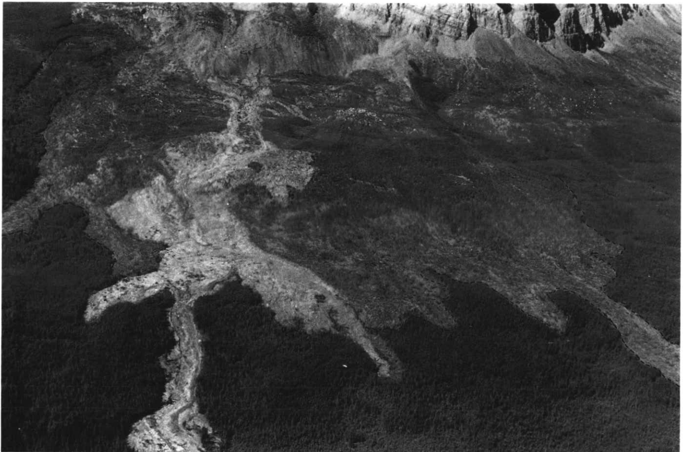
Figure 13 Oblique view of the landslide complex noted in Figure 11. The boundary of the landslide is indicated by a dotted line. Note the unvegetated track of a multi-lobed mudflow that travelled from the upper part of the complex to the Liard River.
