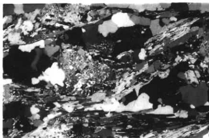
Figure 3 Optical photomicrograph of muscovite and biotite as retrograde metamorphic products in a reworked Archean basement gneiss below the basal décollement. The phyllosilicates define a C/S fabric (horizontal C-planes, S-planes dipping to the left) which indicates a top-to-the-south sense of displacement for the rocks. Sample collected northwest of lac Watts just below the basement-cover contact.
