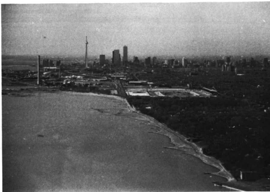
Figure 8 View looking west of the Eastern Beaches (Fig. 2) toward the downtown core showing groyne and resulting entrapment of littoral sediment transported by the long shore drift system
