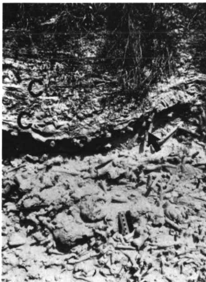
Figure 10 Modern hard laminated caliche (C) developed on soft Pleistocene reef limestone, Barbados (scale in cm)
