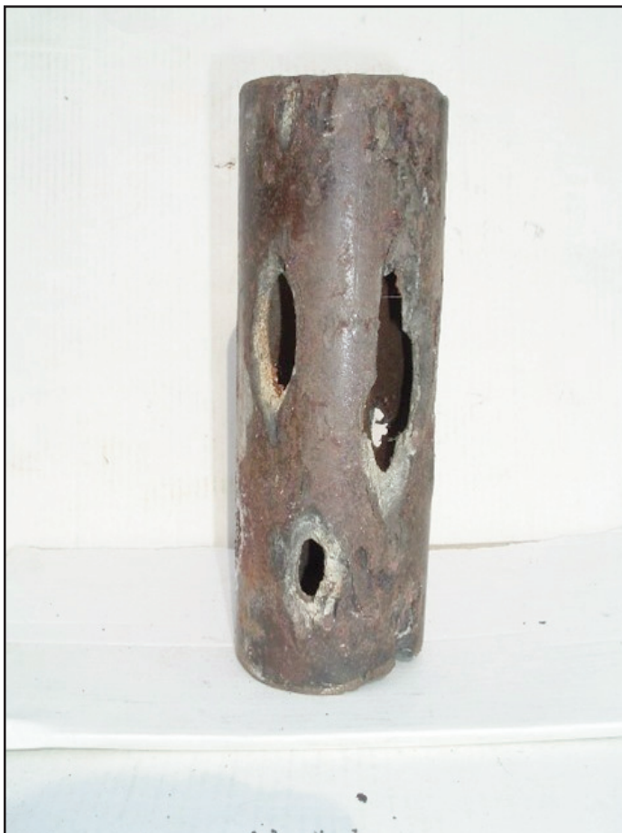
Figure 6. Production tubing (7.3 cm diameter) from the Morpeth gas field showing corrosion due to hydrogen sulphide.
