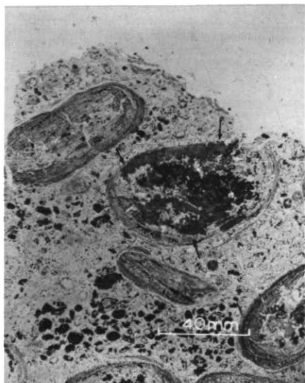
Figure 6. Oolitic and pisolitic iron formation. Concentric texture of pisolites is beautifully preserved by submicroscopic crystallites of hematite. Carbonate porphyroblasts (probably siderite, dark grey shown by arrows) destroy the concentric texture. Thus, this is a hematite facies rock, overprinted by younger carbonate facies. Section B13-10, Labrador trough.
