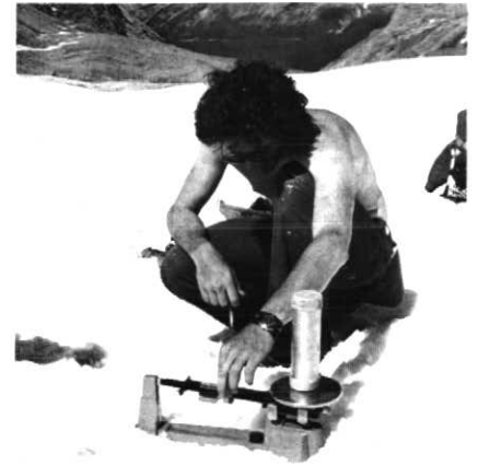
Figure 1 Snow density determination, Peyto Glacier.
