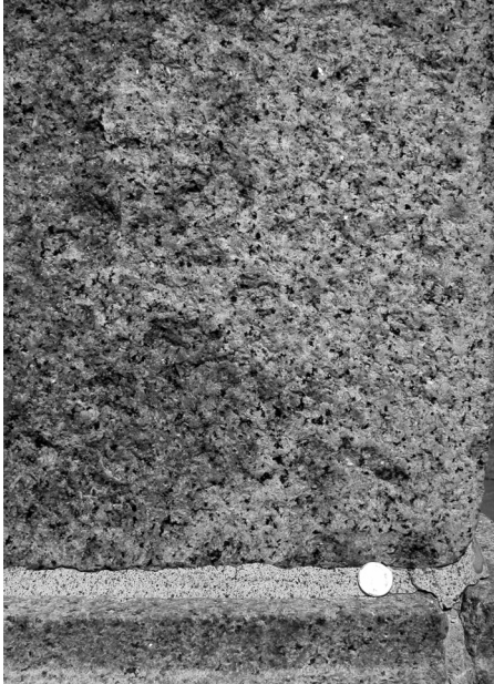
Figure 5 Close-up photograph of the Leinster granite base of the statue of the Immaculate Conception. The stone is a dark grey, medium- to coarse-grained, undeformed hornblende tonalite or quartz diorite. Quarter for scale.
