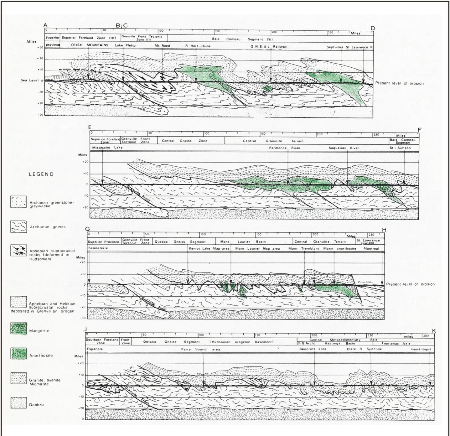
**Figure 7.** Schematic orogen-scale cross-sections through the Grenville Orogen (from Wynne-Edwards 1972). A–D Eastern Québec; E–F Central Québec; G–H western Québec; J–K southern Ontario. Note the recognition of NW vergence and inferred crustal scale of the Grenville Front. A feature of all the cross-sections is the inferred presence of Archean basement overlain by remnants of Proterozoic passive margin supracrustal sequences of various ages (the basement–cover hypothesis).
