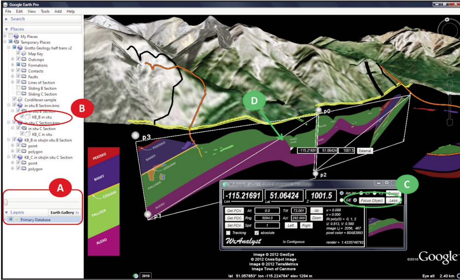
Figure 10. WxAzygy® Tools operating in 3-D on the selected COLLADA cross-section. The WxAzygy® interface provides the ability to ‘point and click’ on a COLLADA surface without leaving Google Earth®. This add-on uses the GE COM API to interpret a user click event on the GE surface as an intersection with a COLLADA model along the user’s line of sight. Note that the coordinates of the selected point provide the real world location {long, lat} and height {metres} above the geoid, which, in this example, is below ground level. The ability to remove the Primary Database (A) is currently supported only in Google Earth® 5.x and 6.0. In version 6.2, the Radar item in the Weather folder must be made transparent. User highlights the COLLADA surface (B), then selects that surface as the Focus Layer (C) and uses the geoCursor (D) to click on that surface (©2012 Google, GeoEye, TerraMetrics, and Cnes/Spot Image).
