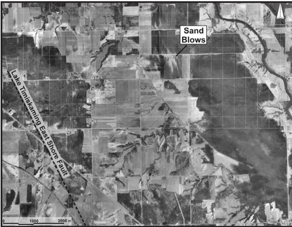
Figure 8. Lighter toned ‘sand blows’ on the floor of the Little Clay plain northeast of New Liskeard, where liquefied sand has been injected up through overlying darker peats during seismic activity. These remain to be investigated by trenching. See Figure 4A for location.
