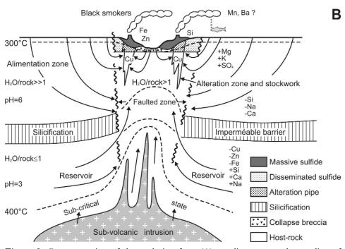
**Figure 2.** Representation of the evolution from (A) a rudimentary understanding of massive volcanogenic sulfide deposition (Guilbert and Park 1986), to (B) a predictive model of an exhalative system that integrates source, transportation and deposition (Eckstrand et al. 1995).
