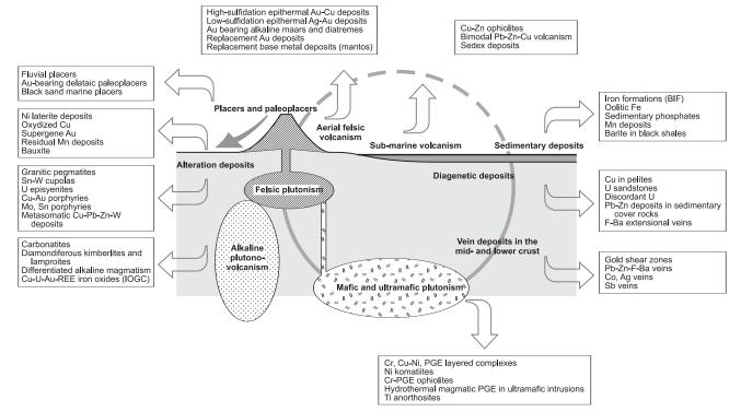
**Figure 4.** Positions of the main deposit types according to the rock cycle. Not to scale.
