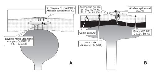
Figure 3. Examples of mineralization associated with an emerging hot spot. (A) oceanic environment; (B) continental environment.
