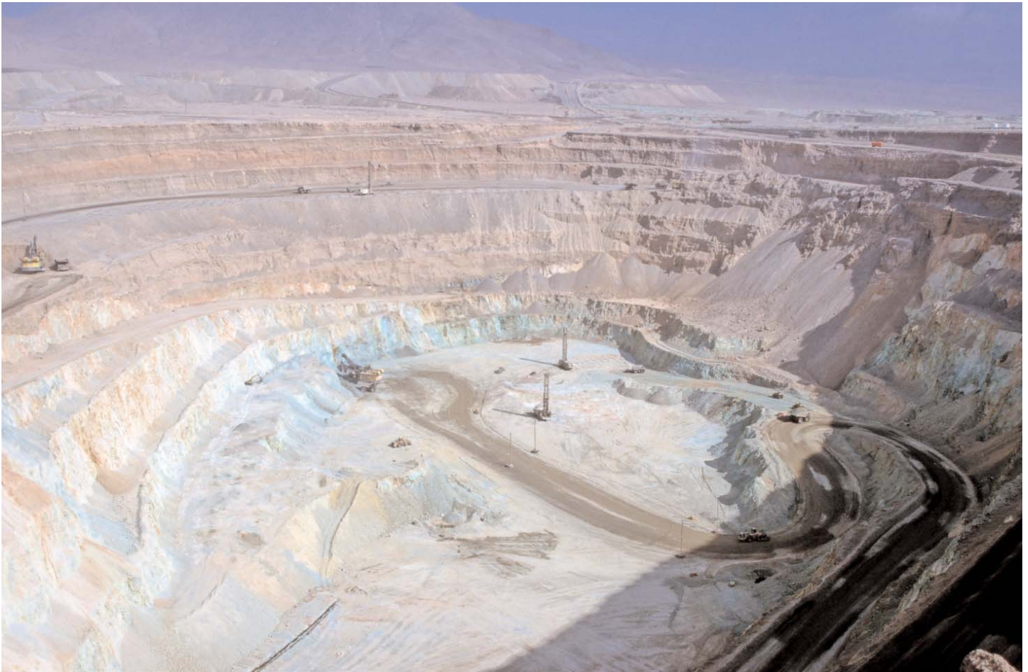
Figure 10. View of the Radomiro Tomic deposit pit, in February 1999, showing the upper part of the oxide zone covered by a variable thickness of piedmont gravels. Green colour is atacamite.
