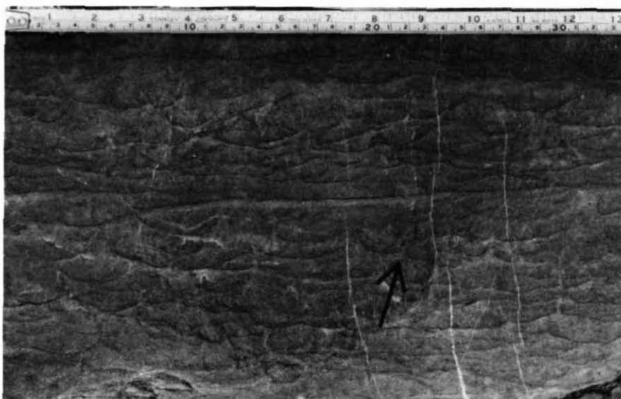
Figure 7 "Dish" structures, formed by rapid dewatering of a massive sandstone. Some of the dish edges curve upward into vertical
