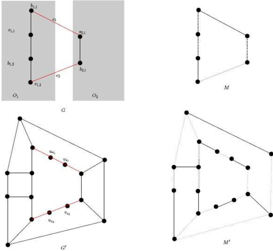
Fig. 3. Construction of  $G'$  and perfect matching  $M'$  from  $G$  and matching  $M$ .
